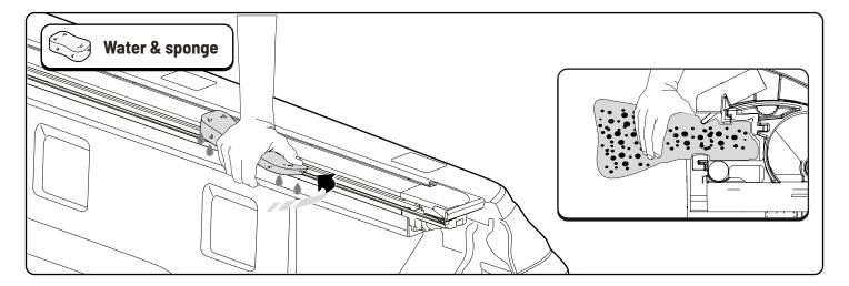
• Clean the drainage channels on the side profiles.
