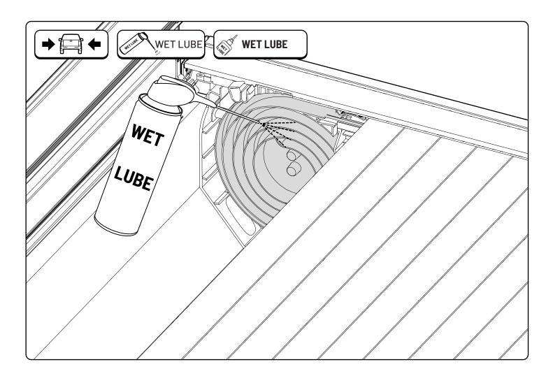
Regularly, and following cleaning, apply a PTFE-free all-conditions wet lube product to the inside of the canister ends.
