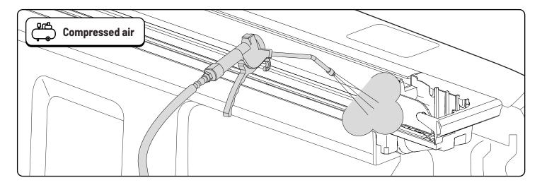
Remove dirt and debris using compressed air.
