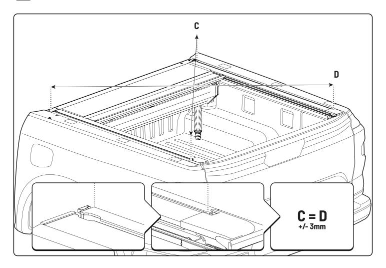
• Ensure the cross measurements are identical.
